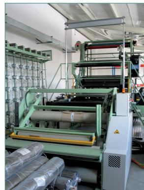
Fig. 5: Biaxial machine, used for basalt UD-tape production.
