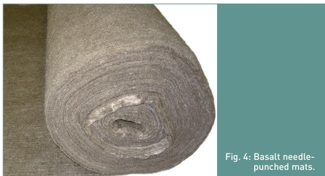
Fig. 4: Basalt needle-punched mats.
