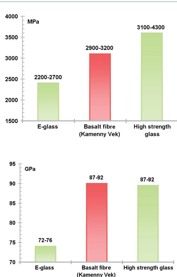
Fig. 2: Properties of basalt and glass impregnated strand [ASTM D2343]
