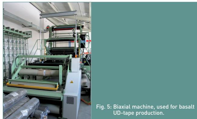
Fig. 5: Biaxial machine, used for basalt UD-tape production.
