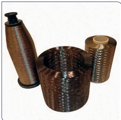
Fig. 5: 2400-tex direct roving for pultrusion compared with assembled roving and twisted yarn
