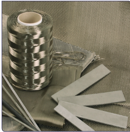
Fig.3: Composite panels and fabric made with Basfiber
