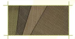
Basalt fabrics are produced from high-quality rovings or twisted yarns and have different weave types and surface densities.
